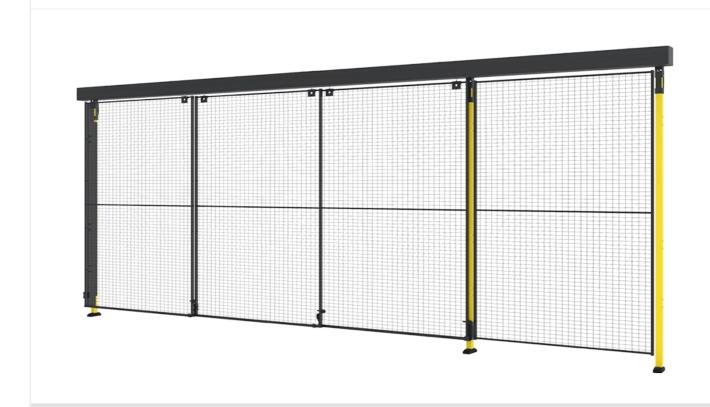
The X-Guard triple telescopic sliding door is designed for industrial settings that require a large opening but have limited space for traditional sliding doors. Featuring a 3-step rail system, the panels overlap instead of sliding fully outward, reducing the need for side clearance while maintaining easy access. With a maximum width of 3x1500 mm and a height of 2500 mm, it offers a practical and efficient safety solution.
